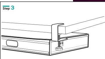
Turn the adjustment knob to secure tightly to desk.
